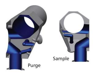
Sample outlet features a reducing ferrule (.75" connection to a .5" port) to maximize drainability of the small diameter port.
