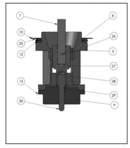
M-Form Valve Plug 1/4" & 3/8" Port Diameters
