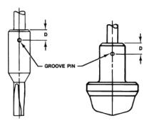
Figure 9. Bolt Torque for Plug/Stem Connection and Plug/Adaptor Connection and Pin Replacement
