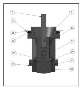
Equal Percentage Valve Plug 1-1/2" & 2" Port Diameters
