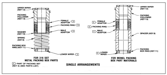
Figure 2: PTFE V-Ring Packing Arrangements for Plain and Extension Bonnets
