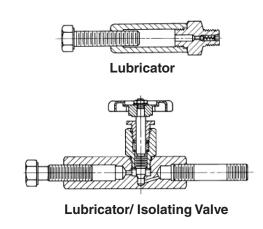
Figure 1: Optional Packing Lubricator and Lubricator/ Isolating Valve
