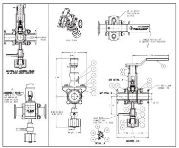
Use PBM's Igenix® Sanitary Block & Bleed Valve to safely isolate the instrument. This valve allows pressure to be vented safely prior to removing the instrument in place.
